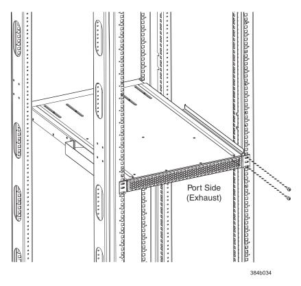
Figure 8. Shelf installed in cabinet
